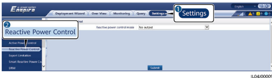
Figure 6-74 Reactive power control
