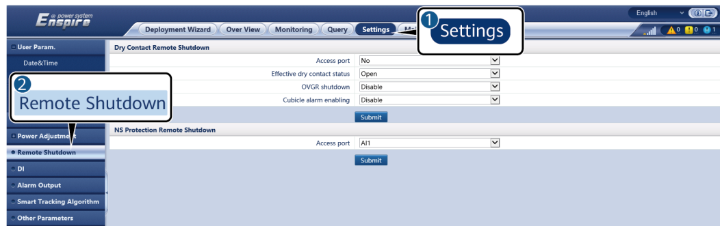
Figure 6-84 Dry contact remote shutdown
