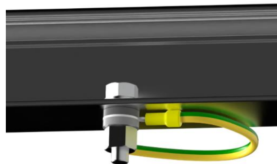
Fig. 11 Grounding of PV modules
