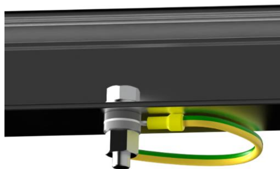
Fig. 11 Grounding of PV modules
